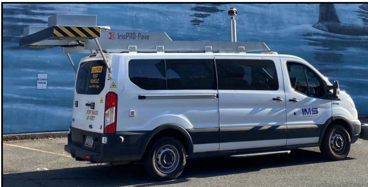
Figure 1 - IMS Integrated Road Information System platform (IRISpro Pavé)
