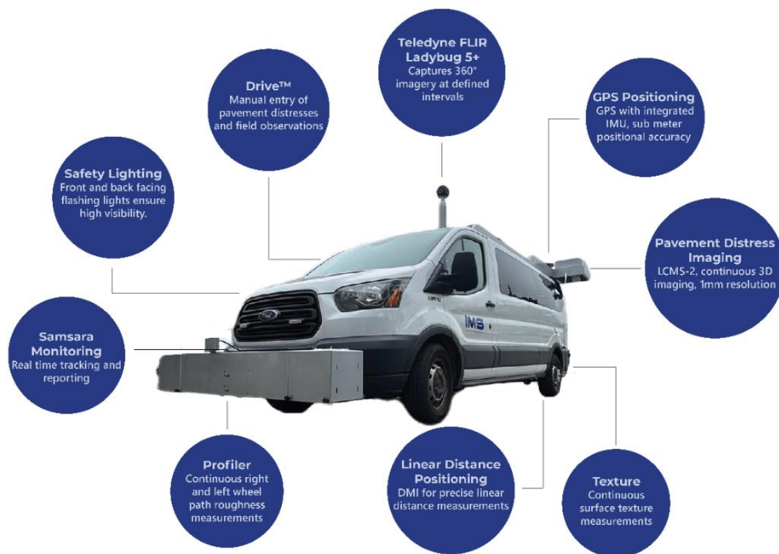
Figure 6 – LCMS-2 data collection vehicle
